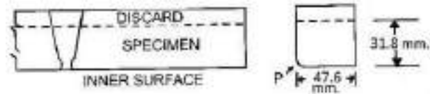
B - REVERSE BEND SPECIMEN
